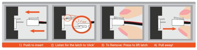
Figure 1: How to Use a JST VH Cable
