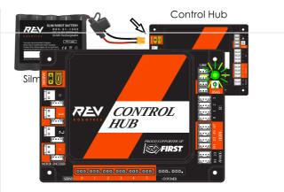
Plug the Control Hub into the PC using a USB-A to USB-C Cable (REV-11-1232)
