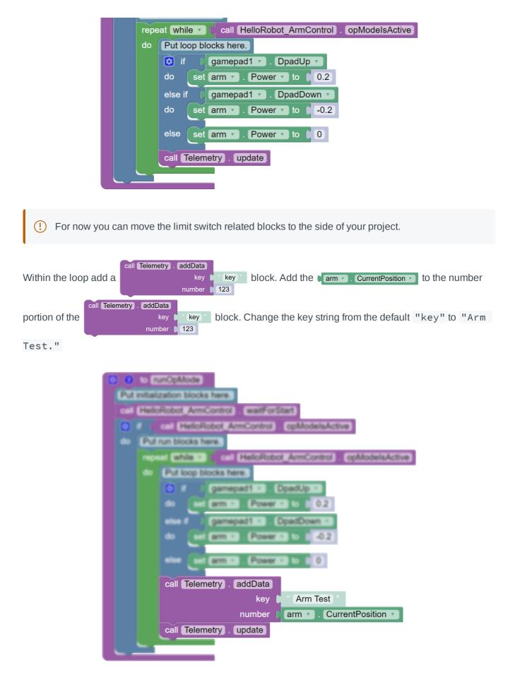
Save the op mode and run it. Use the gamepad commands to move the arm to the 90 degree position. Once you have the arm properly positioned read the telemetry off the Driver Station to determine the encoder count relative to the position of the arm.
