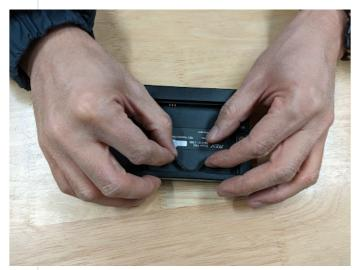
3. Stick foam strip in the middle, both side to side and top to bottom, of the vertical surface opposite the battery contact switch.
