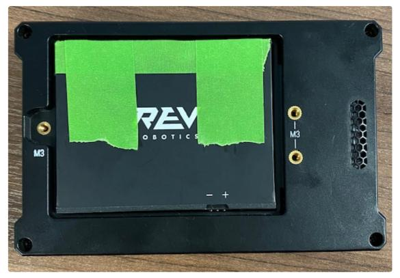
Tape (painters tape or masking tape) is placed on the thin edge above the battery on the side opposite the contacts
