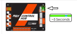
When the OS update has completed, the Control Hub LED will switch from blue, back to its normal blink pattern.
