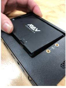
5.2 Continue to push the battery down until it is flush in the case.
