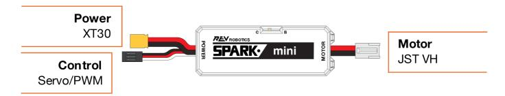
Connect the power wire to a free XT30 port on the REV Control Hub , REV Expansion Hub (REV-31-1153), or through an XT30 Power Distribution Block (REV-31-1293) that is connected to a free Control/Expansion
