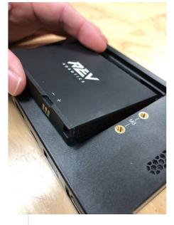
5.1 Insert battery by inserting top of battery towards foam, and gently squeezing battery towards foam with thumb until battery can easily drop into battery case.
